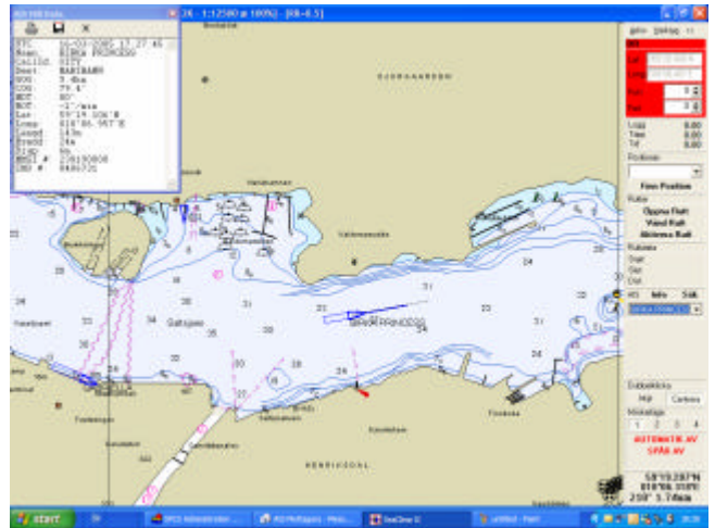
Example how AIS can be presented in a Electronic Chart System
